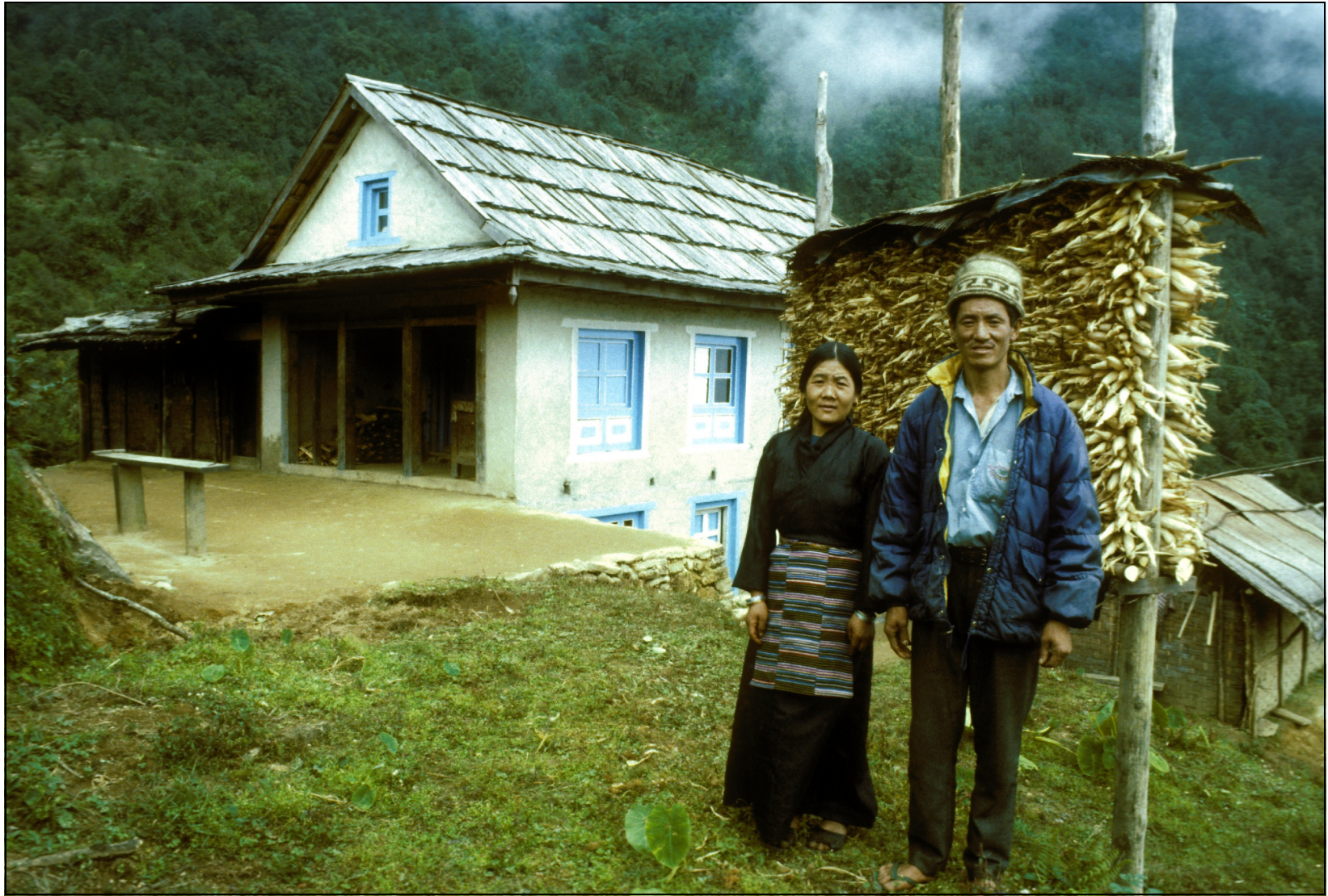
FIGURE 2.2. Modern timber-and-stone home built primarily of Michelia kisopa timber, Castanopsis hystrix roof shakes, and locally-quarried stone.
